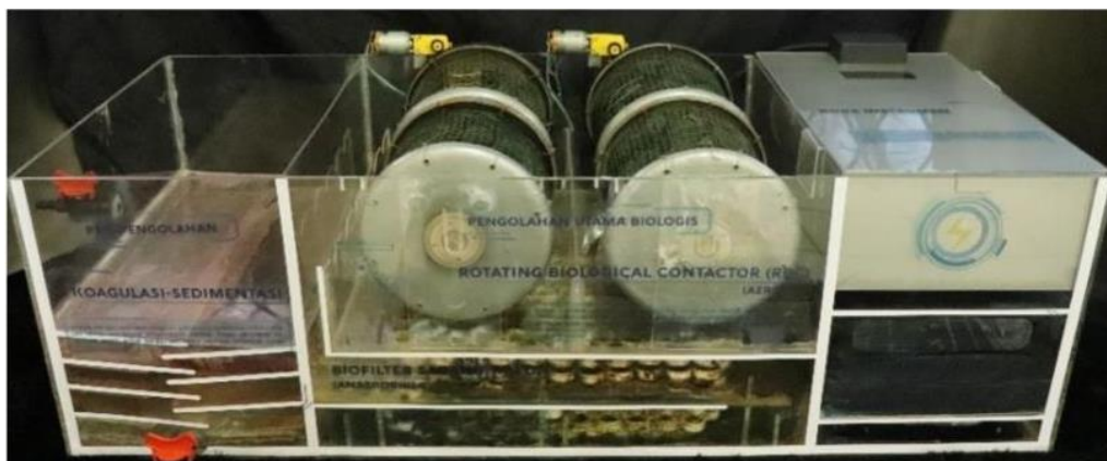
Gambar 1. Reaktor Pengolahan Limbah Cair Tekstil Berbasis Hybrid Attached Growth Biofilm Terintegrasi Arduino (Rahmadi et al. (2022)).
